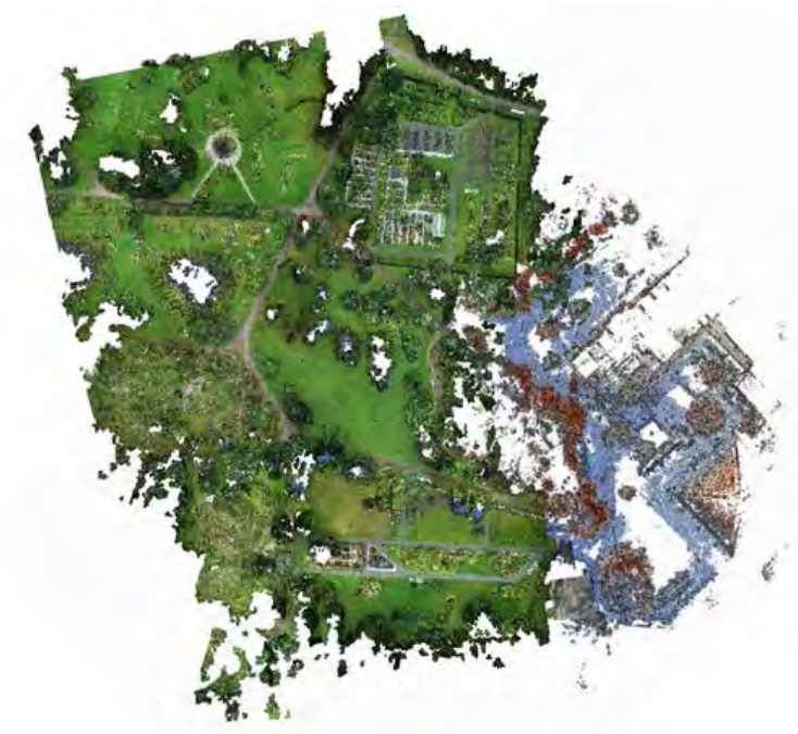
Figure 8. Overlay of UAV and UGV maps. Source: TRADR
