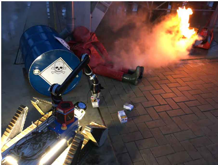
Figure 3: Illustration of the T-Eval exercise environment, the UGVs in action in the Deltalingq training facilities (top) and the UGV extracting a TRADR sample using the arm, near a (dummy) victim, fire and a barrel with chemical substance (bottom).
