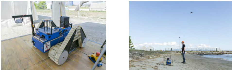
Figure 8: European Robotics League Challenge - TRADR UGV equipped with RTK GPS receiver, payload releaser, and wireless safety switch (left), exploring the competition area together with Jay (right).
