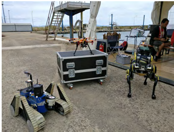
Figure 7: European Robotics League Challenge - Land and Air Robots: TRADR and ANYmal (UGVs), and Jay (UAV).
