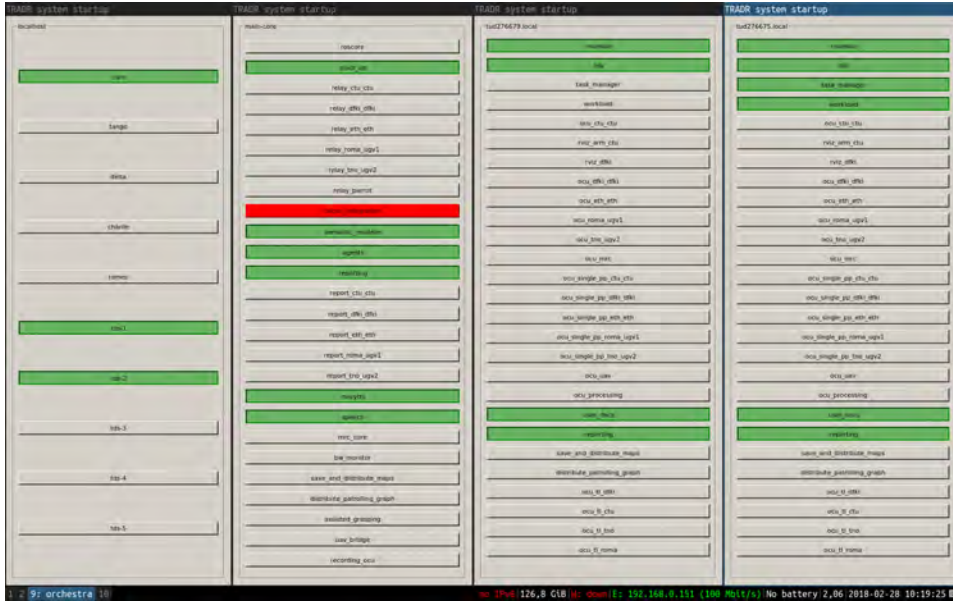
Figure 3: Orchestra provides a visualization of the current system status and is used to start and stop single components.
