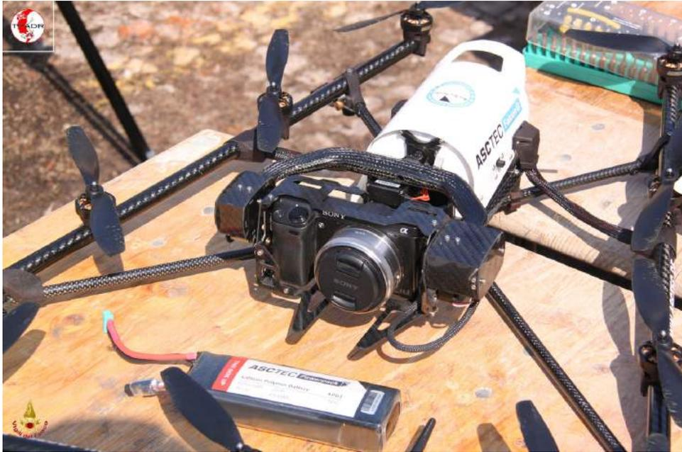
Figure 11: AscTec Falcon 8 equipped with optical camera at Amatrice.
