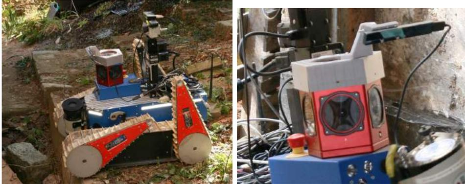
Figure 13: Left: All four flippers equipped with tactile sensing. Right: 3D printed RealSense holder mounted at the top of the Ladybug 3 camera.
