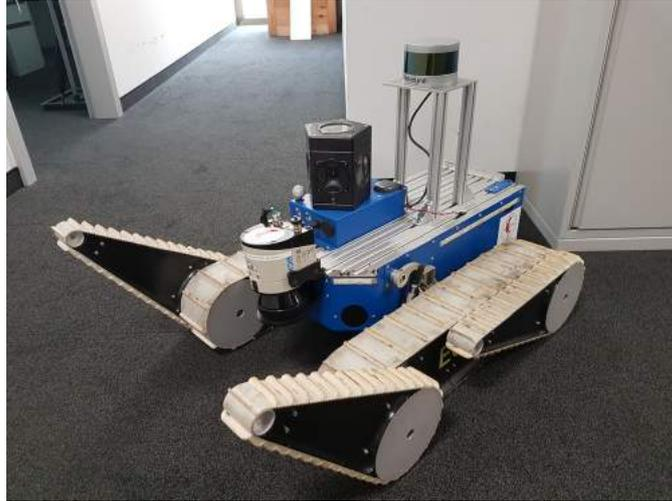
Figure 15: The Velodyne PUCK integrated to the TRADR UGV platform. It is mounted high in order to augment its field of view and localization capabilities.
