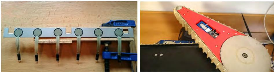
Figure 16: Upgrading flippers. Left: force sensors integrated into a thin metal construction. Right: Upgraded flippers integrates necessary electronics including a radio module.
