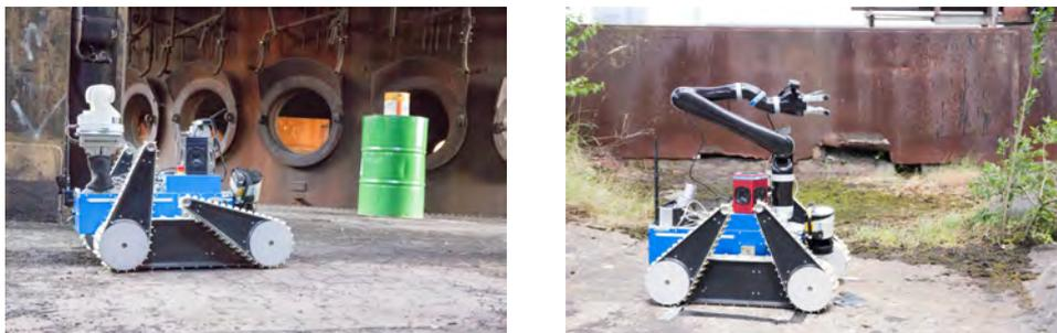
Figure 15: UGV variants. Left: Additional pan-tilt-zoom camera mounted. Right: Kinova JACO arm mounted.
