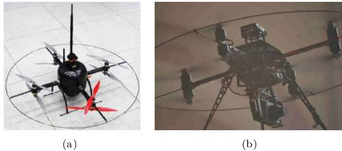
Figure 21. Standard NIFTi UAV octocopter with a standard configuration (a) and NIFTi UAV research octocopter (b) with a camera mounted on top, and a camera in a tilt unit under the main body. Another configuration flow includes a PC and a Kinect-style sensor mounted on top of the research UAV.
