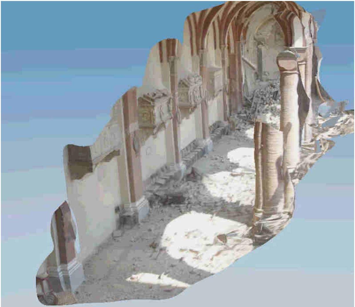
Figure 22. 3D reconstruction based on NIFTi UAV data
