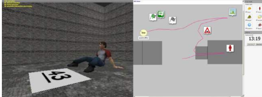
Figure 2: A screen shot of the practice level. The left screen shows the building through the camera mounted on the robot. A victim can be seen, accompanied by a number that could be used to look up information about the victim. The right screen shows the tactical map. The circle on the left corresponds to the location of the robot, the trail to the driven route. Other items shown on the map are (from left to right) a point of interest, a remark, a waypoint, an obstacle, a victim and a picture.
