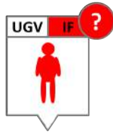
Figure 8. Suggested Design improvement for the ‘explicit unknown’ icon. A source- and destination information is added to make it clearer who is responsible for answering an information request.
