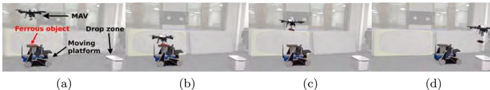
Figure 11: Illustration of the aerial gripping approach. (a) UAV visually servoes above moving UGV, (b) UAV approaches and picks sample from UGV, (c) UAV ascends to operation height, (d) UAV delivers sample to target location.
