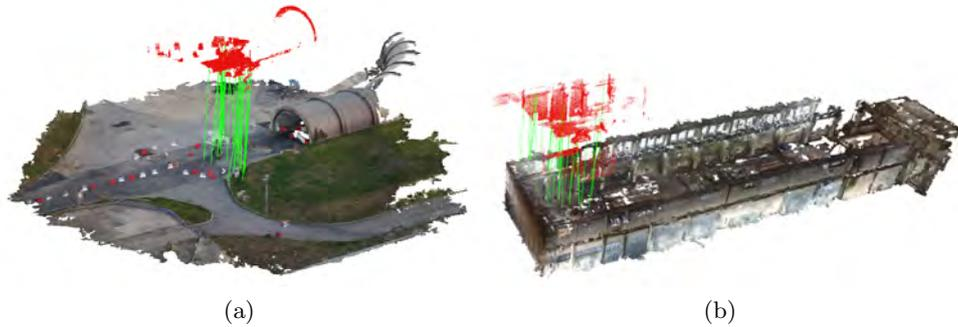
Figure 9: Illustration of the 3D geometric registration approach, a LiDAR point cloud from the UGV (red) is matched against the UAV map (color). (a) Outdoor firemen training site Montebretti, Italy. (b) Indoor Gustav Knepper powerplant in Dortmund, Germany.
