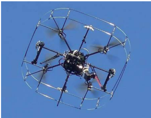
Figure 3: MAV equipped with DGPS, stereo cameras and 3D laser scanner
