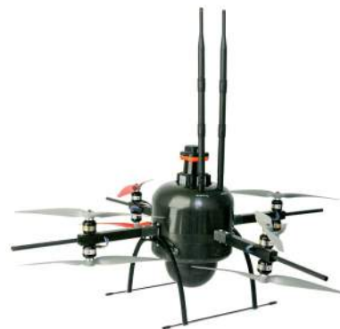
Figure 1: MAV with GPS, laser scanner and camera dome used in rescue operations
