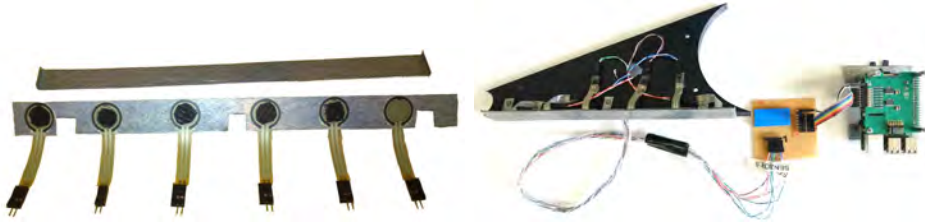
Figure 2: Prototype of the flipper force sensor: array of six sensing elements (FSR 402) is covered by a stripe of steel, forming a thin sensor that fits between the rubber track and the plastic track support. The stripe of steel protects the sensors from the moving rubber track and distributes measured force among them. The sensor is mounted to the plastic track support (top). The sensing elements are passive sensors that exhibit decrease in resistance with applied force. For each sensing element, we use a reference resistor to form a voltage divider and an analog-to-digital converter expansion board for the Raspberry Pi computer to read the six voltages.
