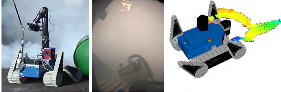
Figure 1: From left: UGV robot approaches smoke area; Example of visual information that the operator sees inside a cloud of smoke: a crop out from the omni-directional camera (middle) and output of the laser range-finder (rainbow-colored point cloud in the right half of the image). Laser beams are randomly reflected by smoke particles. The resulting 3D point cloud is just noise close to the robot.
