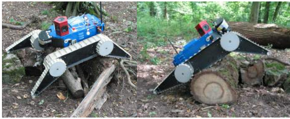
Figure 3: NIFTi UGV Robot climbing capability: Articulated flippers and passive differential increase the platform stability on uneven terrain and enlarge its operability space.
