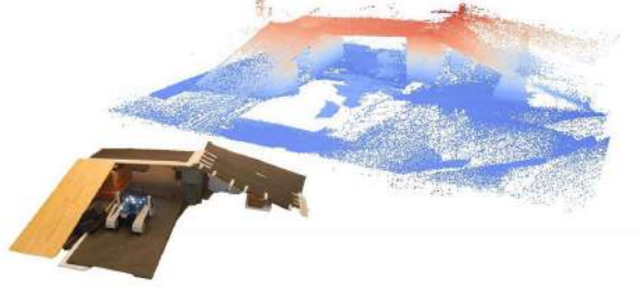
Figure 7: The 3D structure for testing of obstacle traversability shown a metric map created by ICP.
